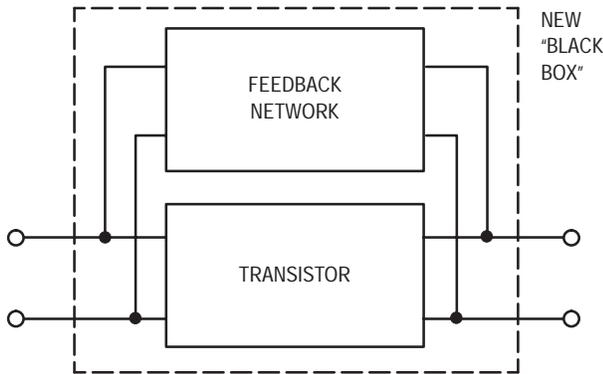
For example, the above combination of transistor and feedback network may be characterized as a single “black box” by the following equations:†
